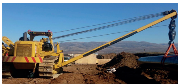
Pipelayers lifting capacity from to 130 Mt
